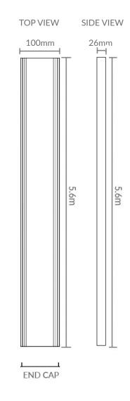
\* Total length of full grate is 5.8m, total usable length is 5.6m to allow for any wastage during the anodising process.
