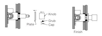
11. Slide plate onto body, position the diverter knob, tighten it with a grub screw using an Allen key, and cap the grub screw hole.
