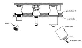
4. Remove the gauge, self-tapping screw, washer, and plastic sleeve in sequence.
