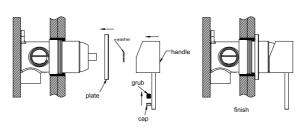
10. Slide plate onto body, attach the washer to the cartridge, position the handle, tighten it with a grub screw using an Allen key, and cap the grub screw hole.
