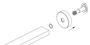
3. Fit the back plate onto the spout adapter.4. Place the ABS washer against the backplate.5. Push the spout onto the spout adapter.
