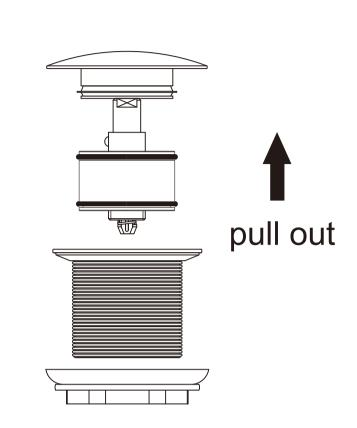
1. Disassemble pop -up waste by pulling out the cap.
