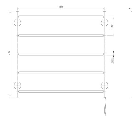
Electricity Input: 240V, 50Hz | Power Rating: 45W | IP Rating: IPX4 | Connection position: Bottom right | Connection type: Plug-in or Hardwire
