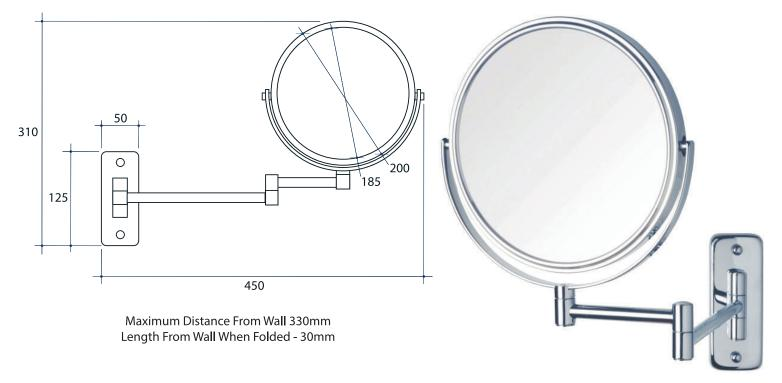
Note: All dimensions are in millimetres (mm)
